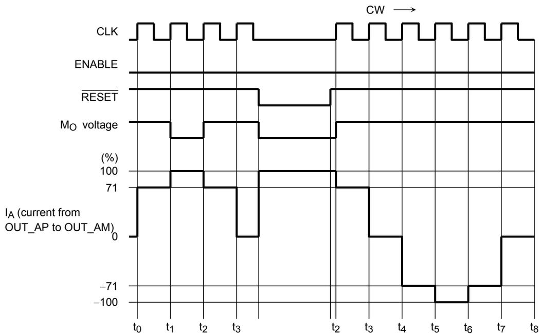
Setting the  $\overline{\text{RESET}}$  signal Low causes the outputs to be put in the Initial state and the  $M_O$  output to be driven Low (Initial state: A-channel output current is at its peak (100%)).
