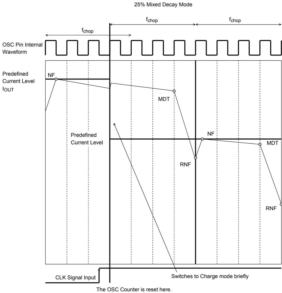
**16. Internal OSC Signal and Output Current Waveform when Predefined Current is Changed from Positive to Negative (when the CLK signal is input using 2-phase excitation)**
