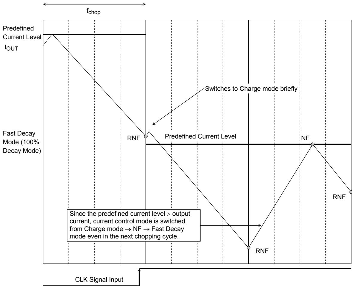
**13. CLK and Internal OSC Signals and Output Current Waveform
