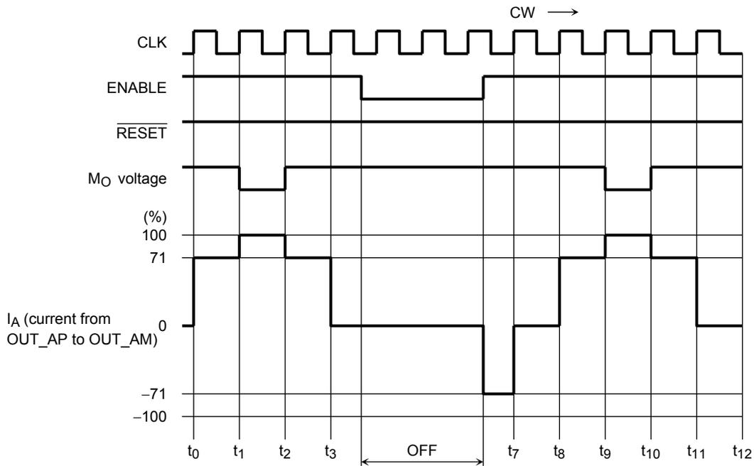
Setting the ENABLE signal Low disables only the output signals, while internal circuitry other than the output block continues to operate in accordance with the CLK input. Therefore, when the ENABLE signal goes High again, the output current generation is restarted as if phases proceeded with the CLK signal.
