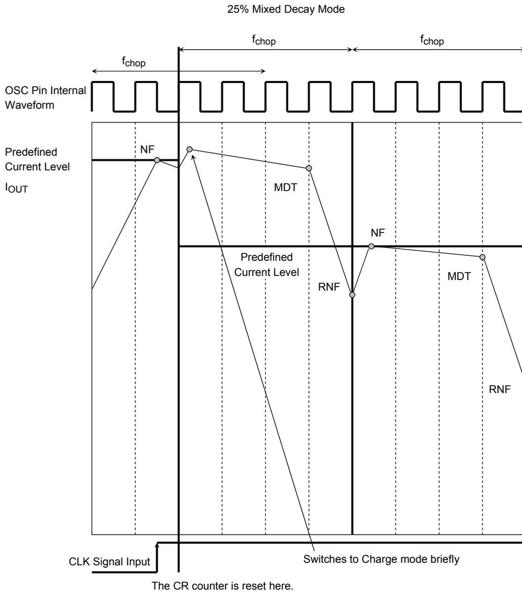
When the CLK signal is asserted, the Chopping Counter (OSC Counter) is forced to reset at the next rising edge of the OSC signal.
