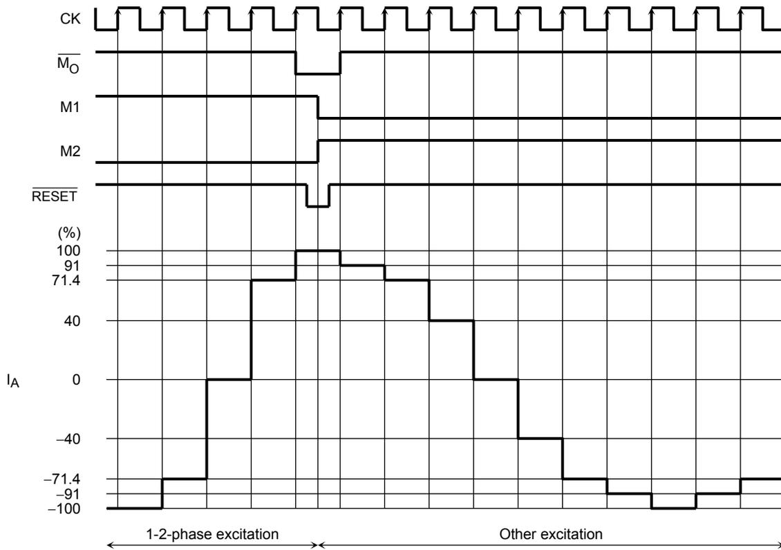
It is recommended that the state of the M1 and M2 pins be changed after setting the  $\overline{\text{RESET}}$  signal Low during the Initial state ( $M_0 = \text{Low}$ ). Even when the  $M_0$  signal is Low, changing the M1 and M2 signals without setting the  $\overline{\text{RESET}}$  signal Low may cause a discontinuity in the current waveform.
