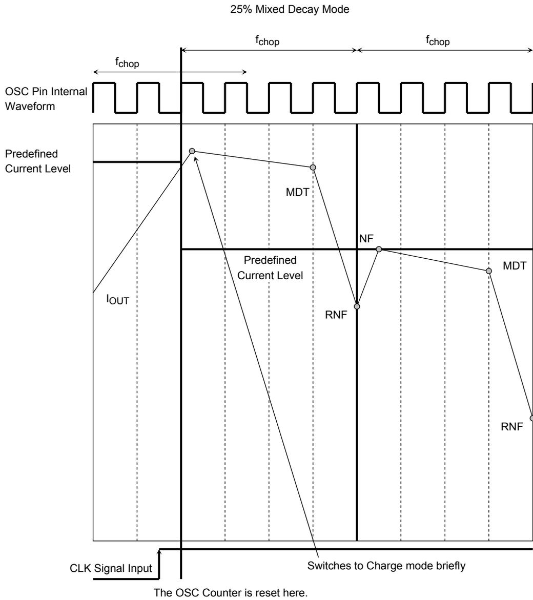
**15. CLK and Internal OSC Signals and Output Current Waveform
