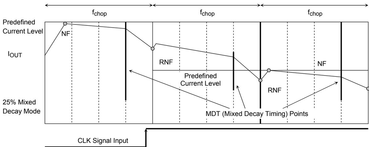
\*: Even if the output current rises above the predefined current at the RNF point, the current control mode is briefly switched to Charge mode for current sensing.
