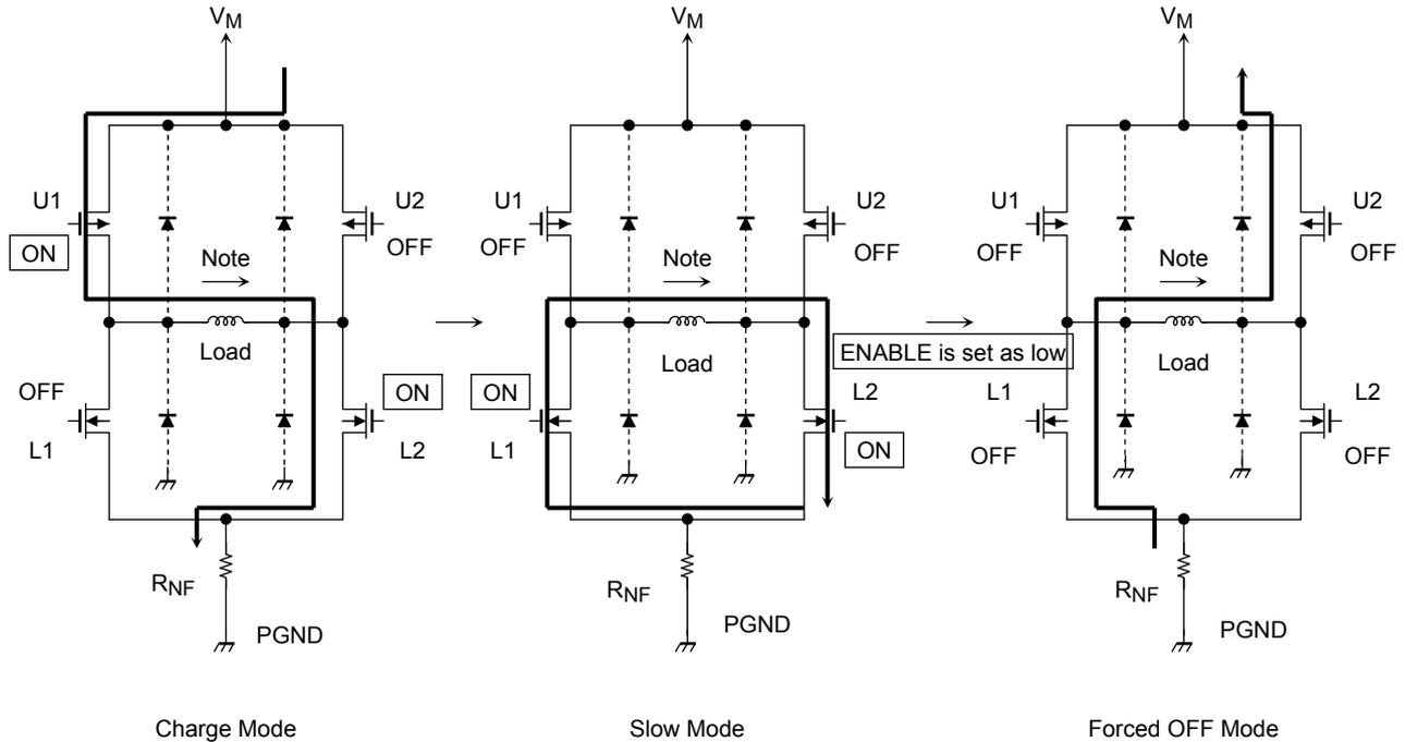
As shown in the figure above, output transistors have parasitic diodes.
