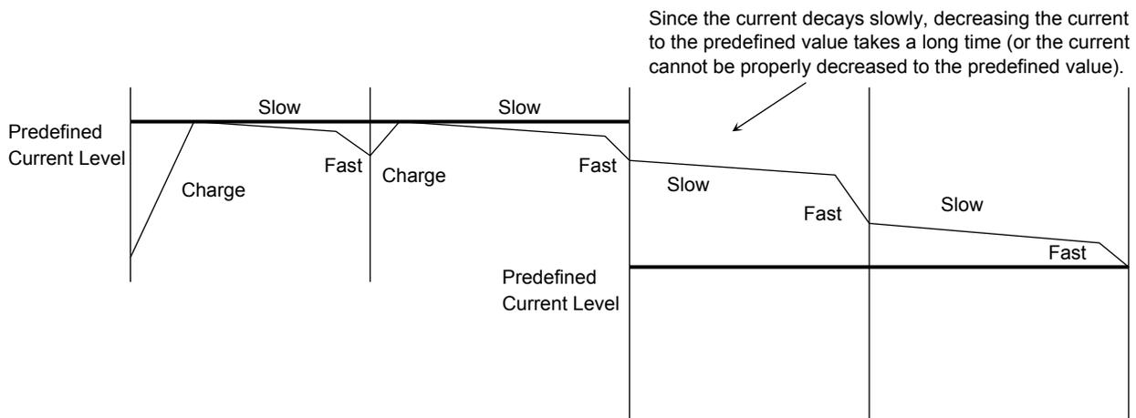
During Mixed Decay and Fast Decay modes, if the predefined current level is less than the output current at the RNF (current monitoring point), the Charge mode in the next chopping cycle will disappear (though the current control mode is briefly switched to Charge mode in actual operations for current sensing) and the current is controlled in Slow and Fast Decay modes (mode switching from Slow Decay mode to Fast Decay mode at the MDT point).
