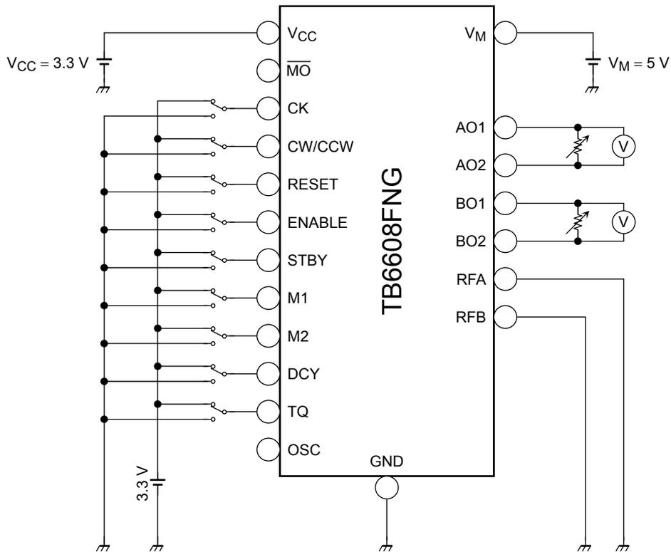
**Test Circuit 5:  $V_{FU}$ ,  $V_{FL}$**
