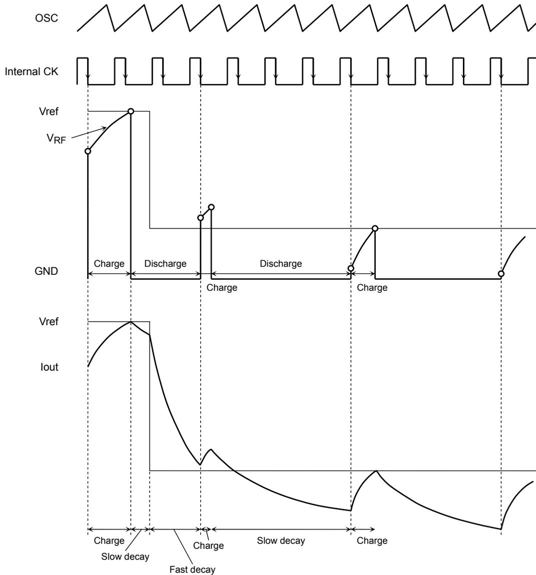
In fast-decay mode, the regenerative current from a coil flows back to the power supply as shown below.
