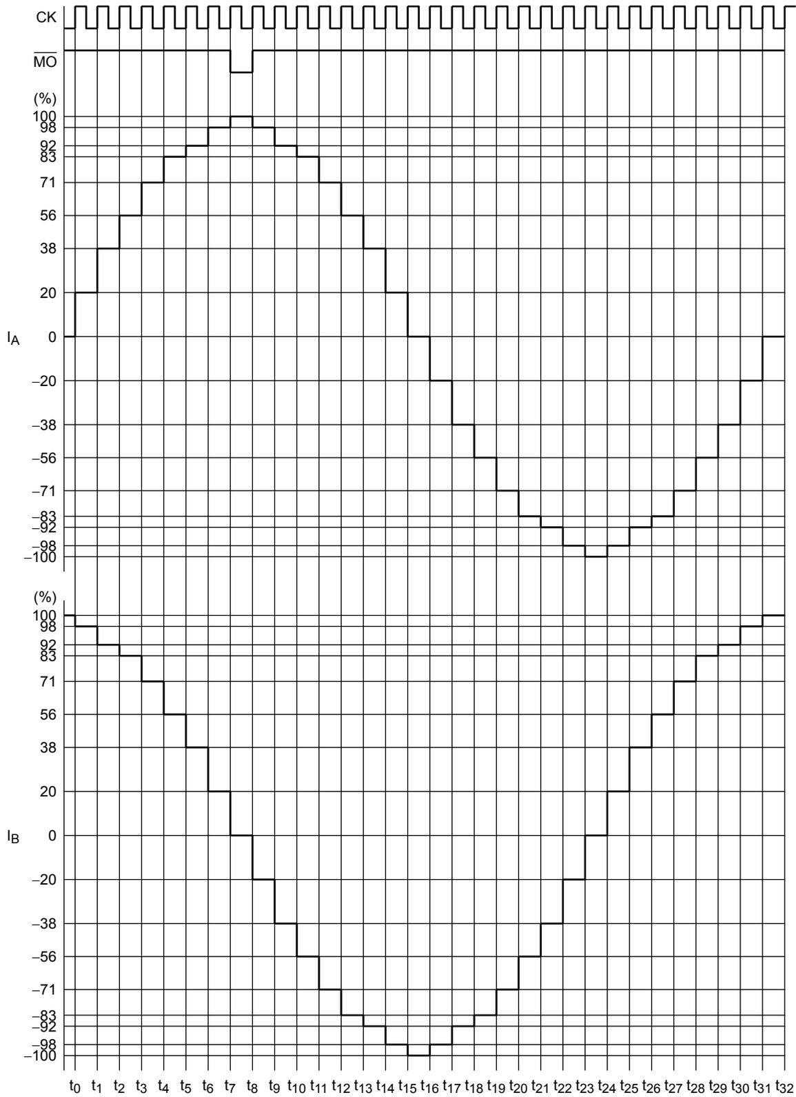
**Output Current Vector Locus (Normalizing a single step to 90 degrees)**
