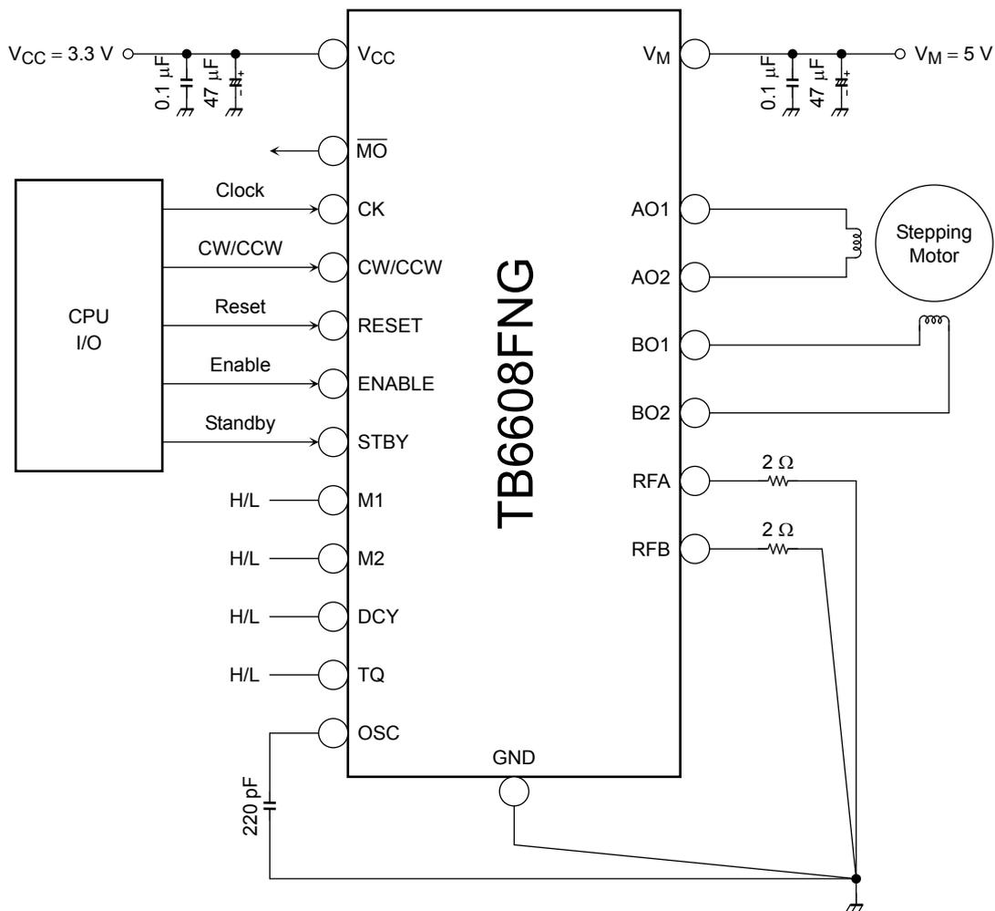
Note 1: Capacitors for the power supply lines should be connected as close to the IC as possible.
