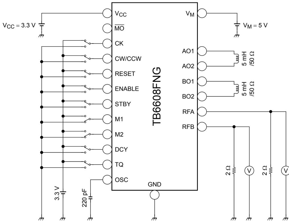
**Test Circuit 4:  $V_{SAT}$  (UL)**
