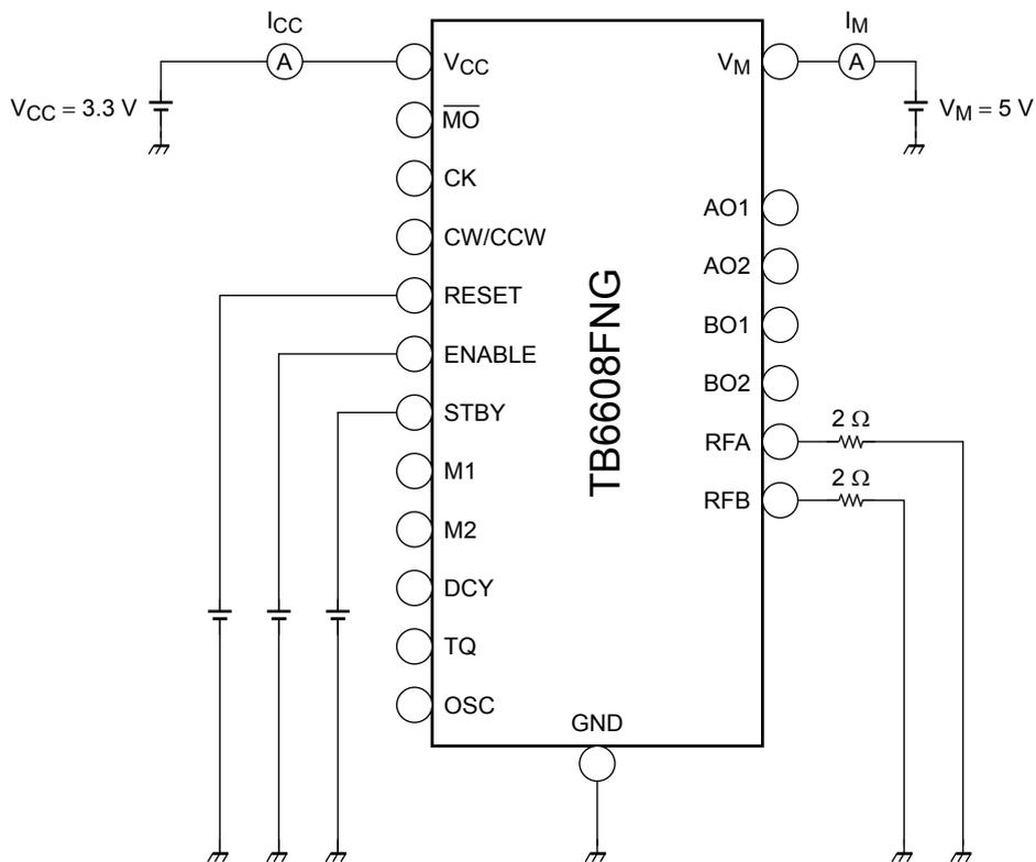
**Test Circuit 3:  $V_{RFA}$ ,  $V_{RFB}$**
