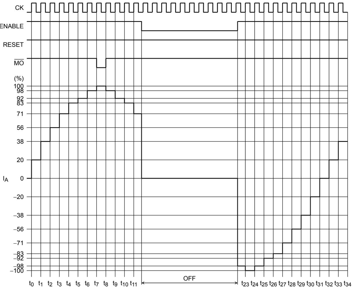
**Relationship between the RESET Input and the Phase Current and  $\overline{MO}$  Outputs**
