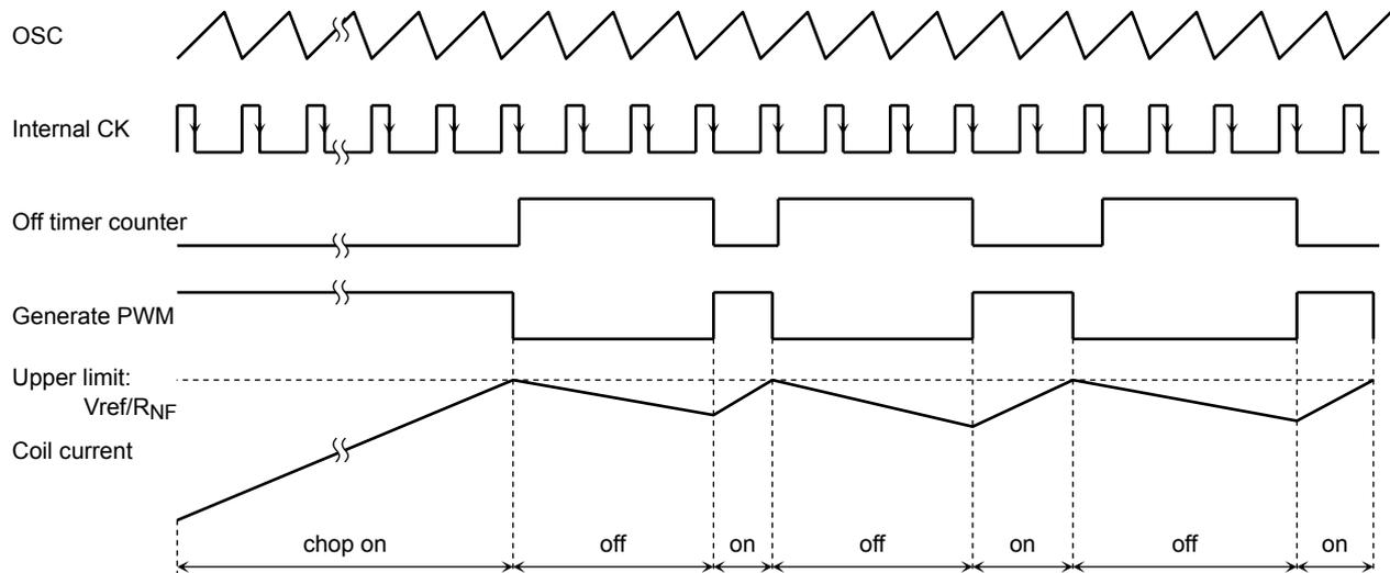
The upper limit of the current across the motor coil (i.e., the peak current in each excitation mode),  $I$  (Limit), can be calculated as follows:
