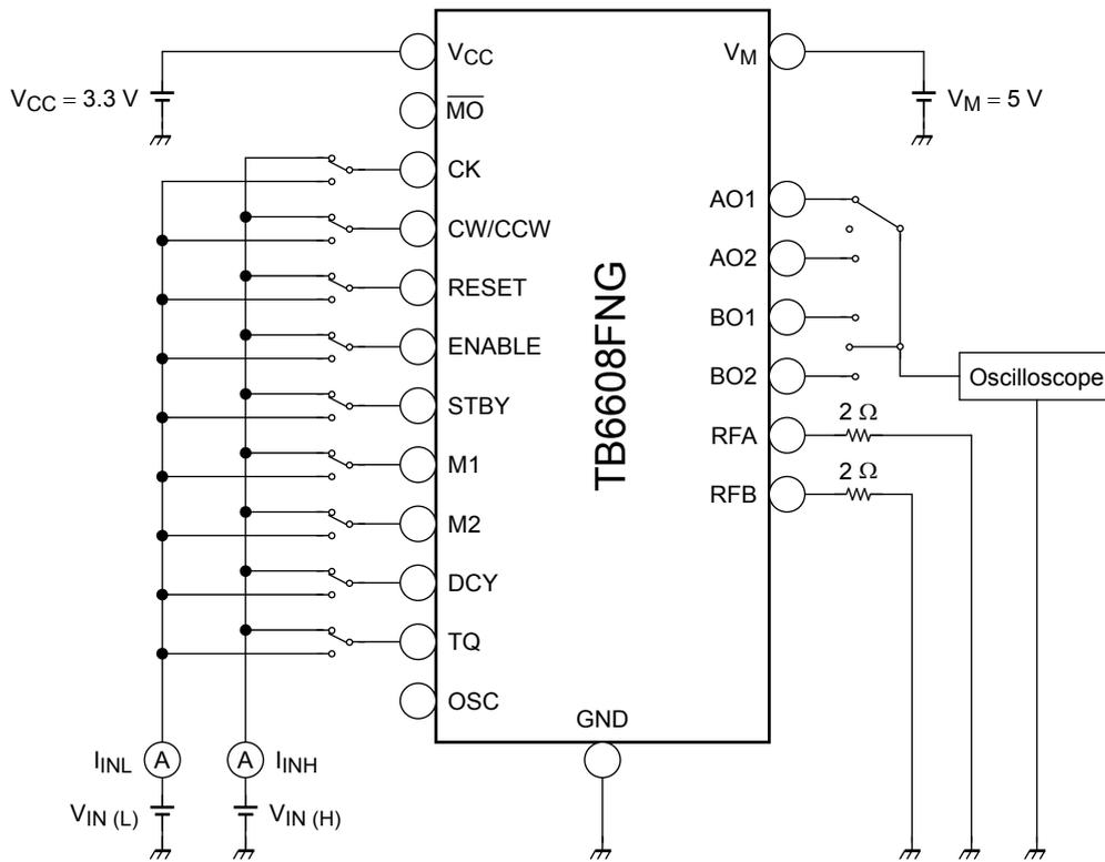
**Test Circuit 2:  $I_{CC}$ ,  $I_M$**
