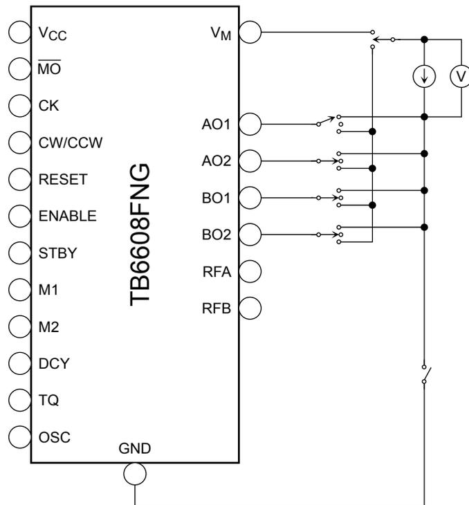
**Test Circuit 6:  $I_{OH}$ ,  $I_{OL}$**
