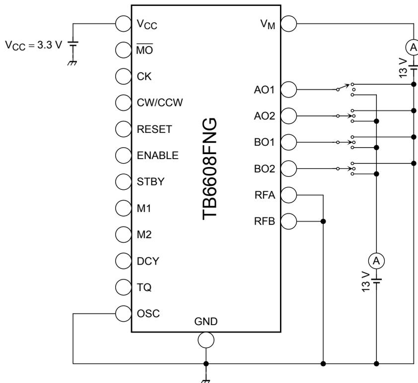
**AC Electrical Characteristics, Test Circuit 7: CK (OSC) and Output Voltage**
